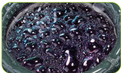
Without A contact angle of max. 95° leads to flat water drops.
