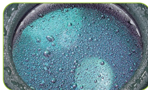
With Contact angles more than 110° lead to ball-like water drops.
